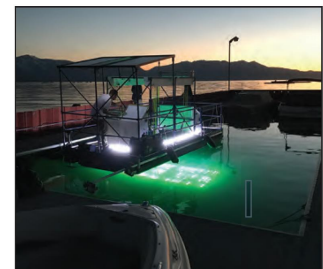
Photo: Inventive Resources, Inc. A boat equipped with ultraviolet light is used to kill aquatic invasive plants at Lakeside Marina.
