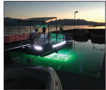
Photo: Inventive Resources, Inc. A boat equipped with ultraviolet light is used to kill aquatic invasive plants at Lakeside Marina.
